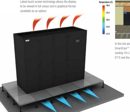
In this hot aisle containment system, three SmartCool™ units, configured as 2 run/1 standby, are cooling 10 x 20kW racks; cold aisle temperature is at 21°C and the hot aisle 36°C
